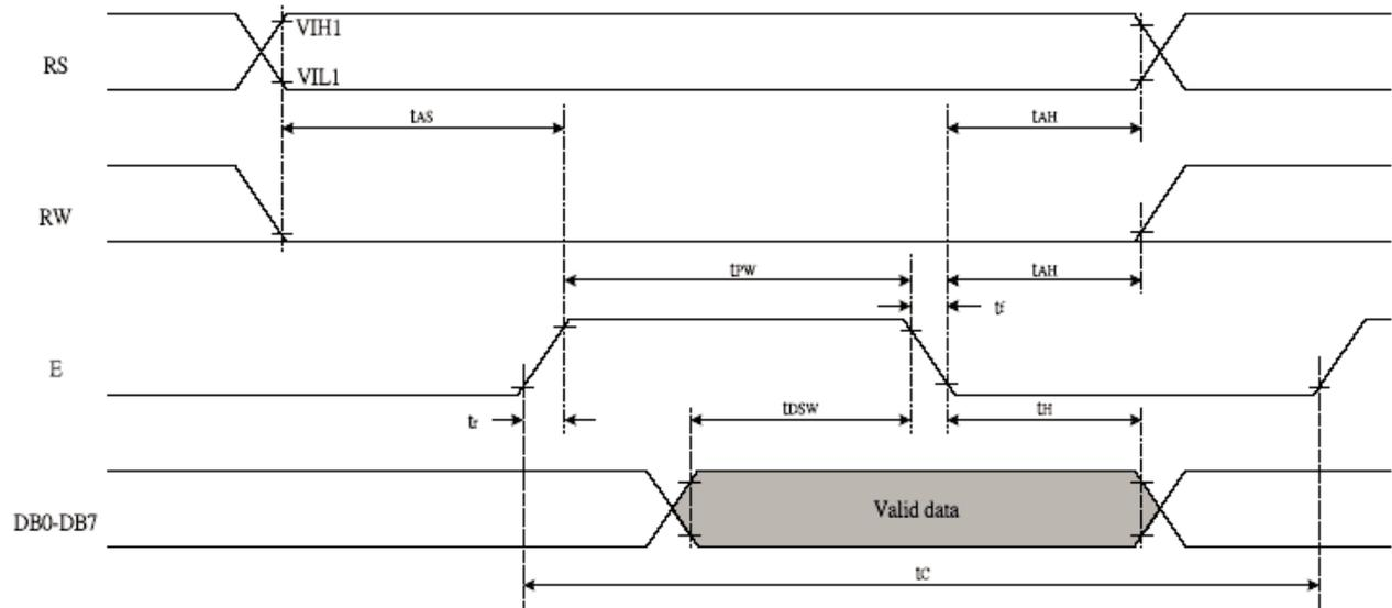
$T_a = -30 \sim +85^\circ\text{C}$ ,  $V_{DD} = 5.0 \pm 0.5\text{V}$
