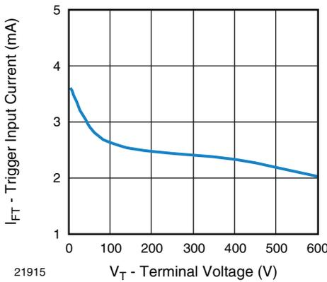
Fig. 12 - Trigger Current vs. V<sub>LOAD</sub>
