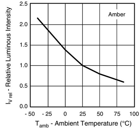
Fig. 7 - Relative Luminous Intensity vs. Ambient Temperature
