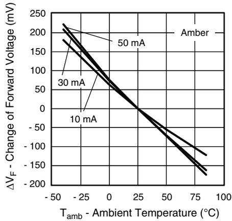
Fig. 9 - Change of Forward Voltage vs. Ambient Temperature
