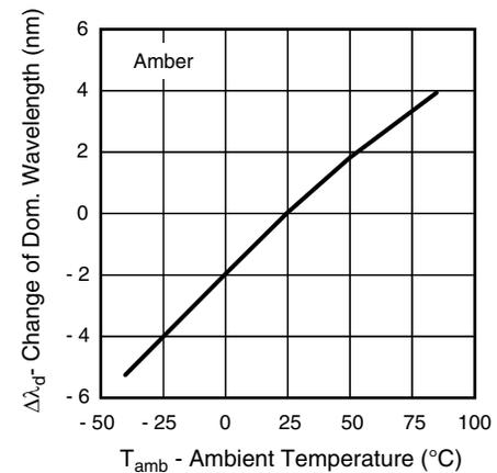
Fig. 8 - Change of Dominant Wavelength vs. Ambient Temperature
