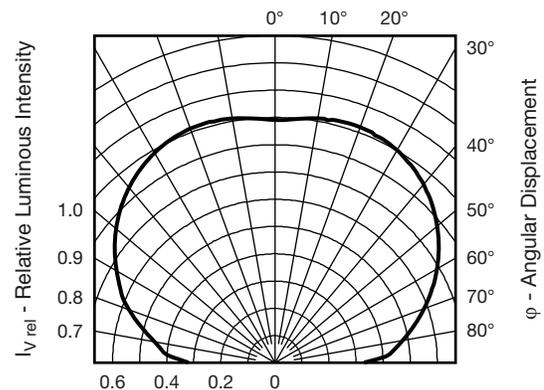
Fig. 2 - Relative Luminous Intensity vs. Angular Displacement
