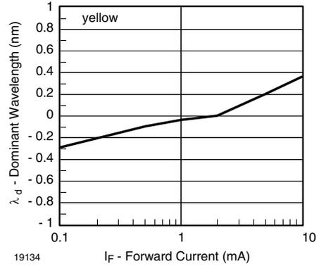
Fig. 6 - Dominant Wavelength vs. Forward Current
