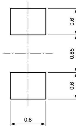
Alternative solder pad, compatible to other 0603 ChipLEDs
