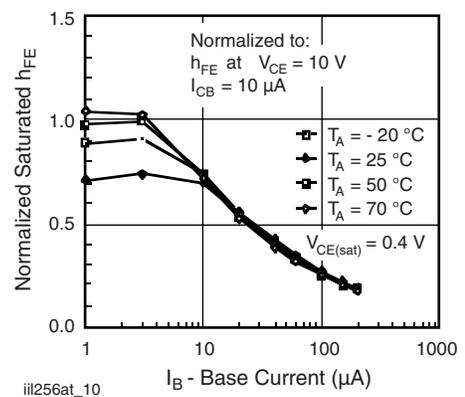
Fig. 10 - Normalized Saturated  $h_{FE}$  vs. Base Current
