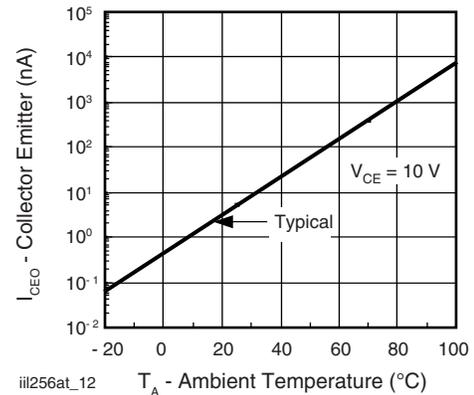
Fig. 12 - Collector Emitter Leakage Current vs. Temperature
