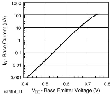
Fig. 11 - Base Emitter Voltage vs. Base Current
