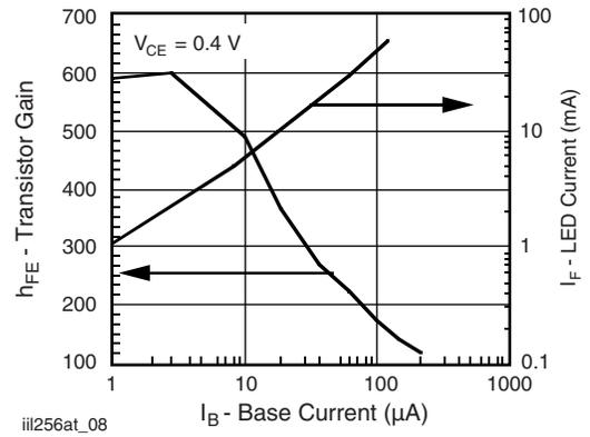
Fig. 8 - Base Current vs.  $I_F$  and  $h_{FE}$
