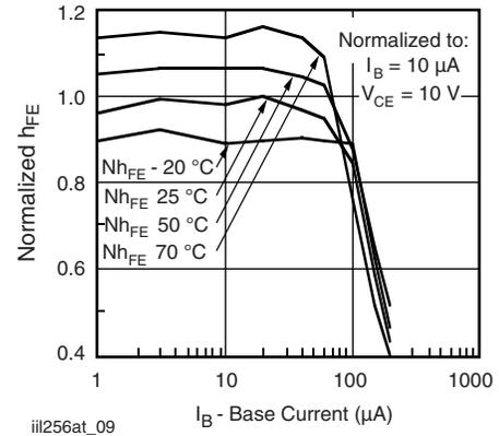
Fig. 9 - Normalized  $h_{FE}$  vs. Base Current and Temperature
