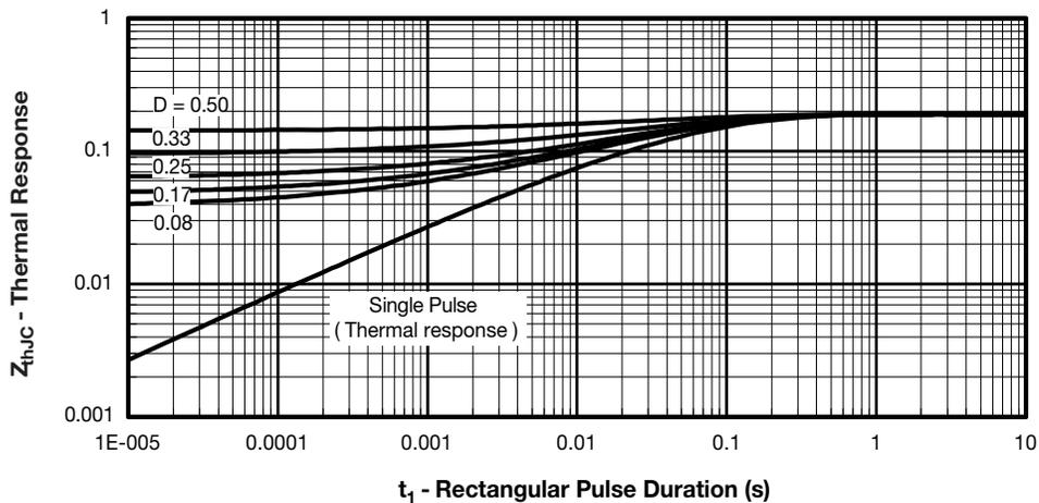
Fig. 9 - Maximum Thermal Impedance  $Z_{thJC}$  Characteristics (Per Leg)
