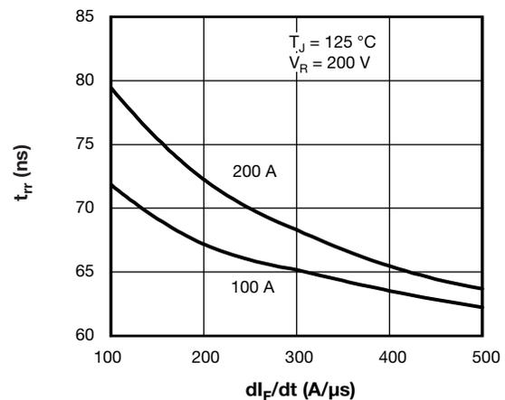
Fig. 4 - Typical Recovery Time vs.  $dI_F/dt$  (Per Leg)
