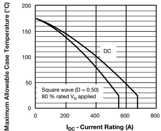
Fig. 3 - Maximum Current Rating Capability (Per Leg)
