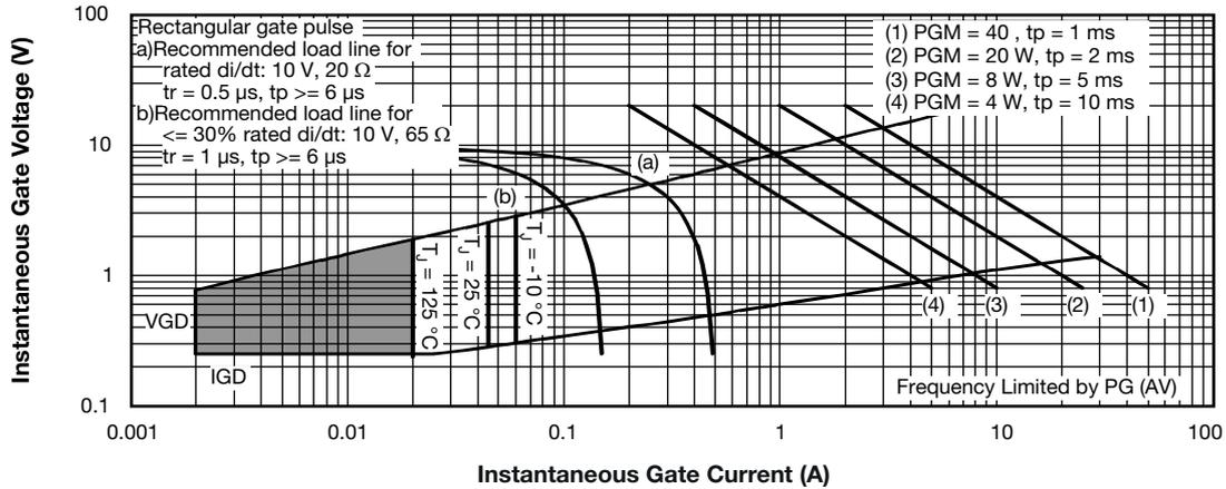
Fig. 9 - Gate Characteristics
