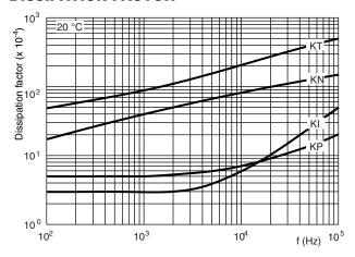
Dissipation factor as a function of frequency at room temperature (typical curve)
