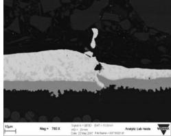
Pic. 1 - Sn-Dot Technology after Pulse Stress
