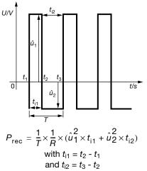
Rectangular pulse with positive voltage amplitude:
