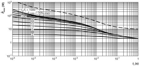
Fig. 2 - Pulse on a regular basis; maximum permissible peak pulse power as a function of pulse duration (*t<sub>i</sub>*)
