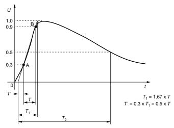
Fig. 5 - 1.2/50 µs or 10/700 µs single high voltage pulse
