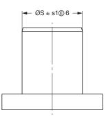
Fig. 4 - Rotor's shaft diameter
