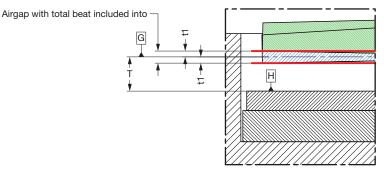
Fig. 7 - Airgap between magnet's top and magnetic cells top
