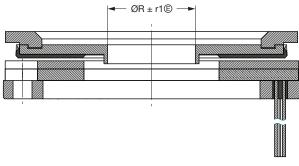
Fig. 3 - Rotor's hole diameter
