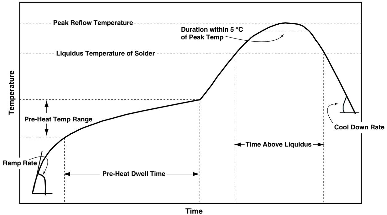
Fig. 1 - Infrared reflow soldering (SMD package)
