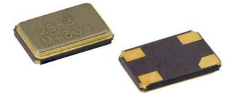
The XT35 is a miniature SMD crystal with 5.0 x 3.2 (mm) ceramic package and a height of 0.8 mm. 12 MHz to 25 MHz frequncy makes it widely applied in PDA, GPS, MP3, and portable instruments.
