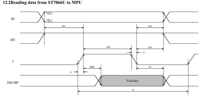
$Ta=-30\sim+85^{\circ}C$ ,  $VDD=5.0\pm0.5V$
