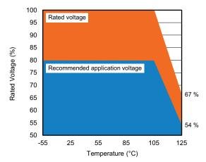
Fig. 1 - Recommended Voltage Derating for Polymer Tantalums
