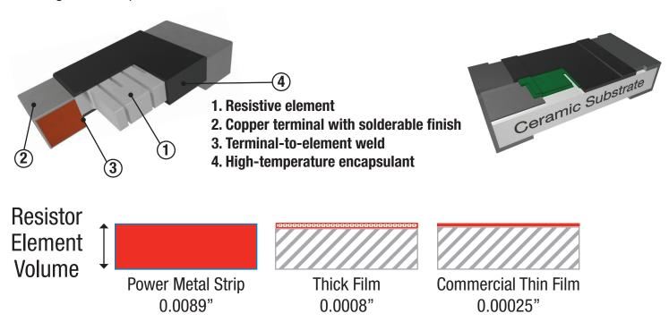
Power Metal Strip resistors are frequently used in applications that experience high-energy, short-term pulse transients:
