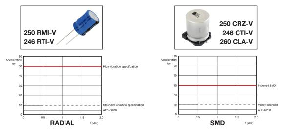
During vibrations, the heavy parts could easily break loose from the PCB. Therefore, care has to be taken in regards to PCB thickness and fixation of the capacitor to the board. Relatively unknown is the appearance of resonances during vibrations. Cases have been reported in which the actual measured vibrational accelerations at the capacitor location gained up to a factor of 50 relative to the pre-set test conditions.
