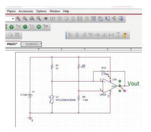
Figure 1. PSpice simulation of Wheatstone bridge for temperature detection
