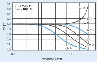
FC series chip resistors are designed with low internal reactance. They function as almost pure resistors on a very high range of frequencies.
