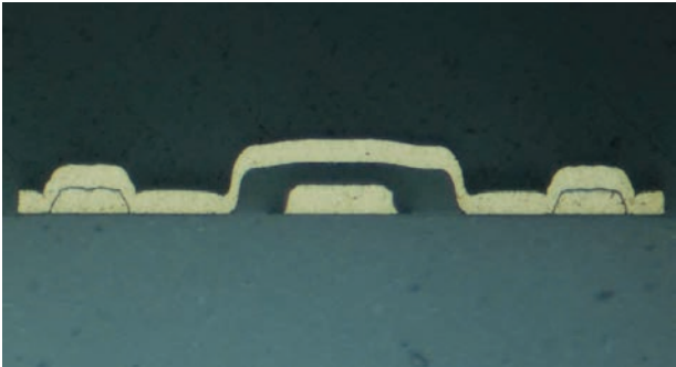
Cross-section of space-qualified polyimide-supported crossover
