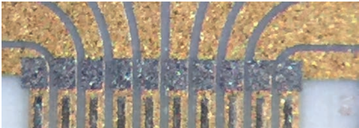
Oxidized TiW Solder dam on BeO device
