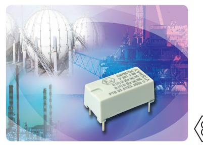
The CNY65Exi provides very high voltage isolation and is ATEX certified per 94/9/EC guidelines for use in potentially explosive environments. The CNY65Exi optocoupler protects equipment and people from being damaged or injured by using infrared light to transmit data and control signals from the typically low-voltage control side to high-voltage equipment.
