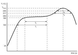
Fig. 5 - Maximum temperature load during reflow soldering
