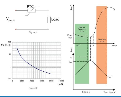
When connected in series with the input of an electrical or electronic circuit load (see Figure 1), such as a small motor or power supply, the PTC thermistor acts as a self-resettable fuse, protecting the circuit against current, voltage and temperature overload conditions.
