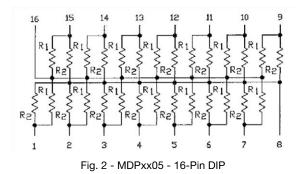
The SIP and the DIP schematics are both basically the same, in that each has two common busses with "N" leads and "N-2" series sets of  $R_1$  and  $R_2$  in parallel between the two busses. This 'unique' electrical schematic makes it impossible to measure the individual  $R_1$  and  $R_2$  values using a simple ohmmeter, a two-wire / four-wire (Kelvin) digital ohmmeter, or a resistance-scanning system without active-guarding capabilities.
