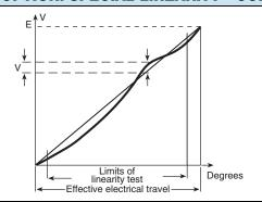
The independent linearity (conformity for the non-linear laws) is the maximum gap  $\Delta V$  between the actual variation curve and the theoretical variation curve the nearest to it. The linearity and the conformity are expressed in percentage of the total applied voltage E
