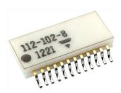
A dual-in-line monolithic ceramic sandwich in a variety of pin sizes (14 to 24) that allow higher resistance integration than traditional chip and wire molded construction. In addition, tighter resistance tolerances can be obtained over traditional molded networks due to the elimination of molding temperature and stress.
