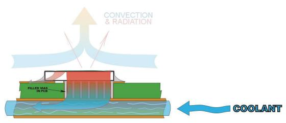
Fig. 5 - Example of Implementing Circulated Coolant Though a Thermal Backplane
