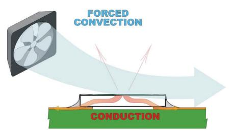
Fig. 6 - Example of Implementing Forced Air Cooling
