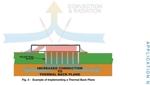
This technique adds higher costs, as the back plane is typically made of heavy copper. In addition, this technique will add weight 🔾
