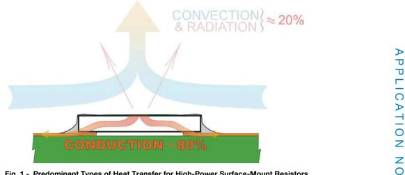
Fig. 1 - Predominant Types of Heat Transfer for High-Power Surface-Mount Resistors
