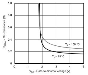
**On-Resistance vs. Gate-to-Source Voltage**
