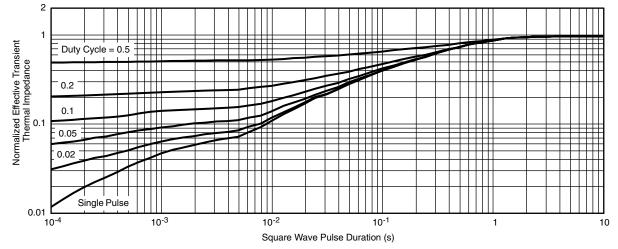
Normalized Thermal Transient Impedance, Junction-to-Case
