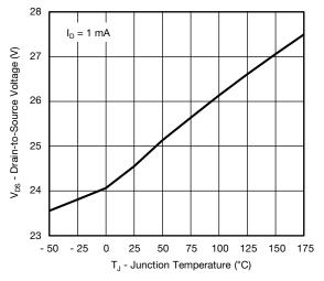
Drain Source Breakdown vs. Junction Temperature
