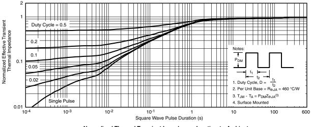
Normalized Thermal Transient Impedance, Junction-to-Ambient
