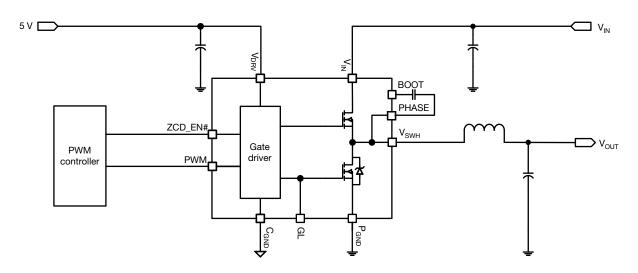
Fig. 1 - SiC544 Typical Application Diagram
