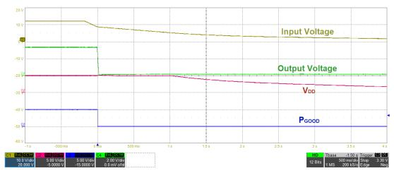
Fig. 16 - Shutdown with V<sub>IN</sub>, No Load (500 ms/div)
