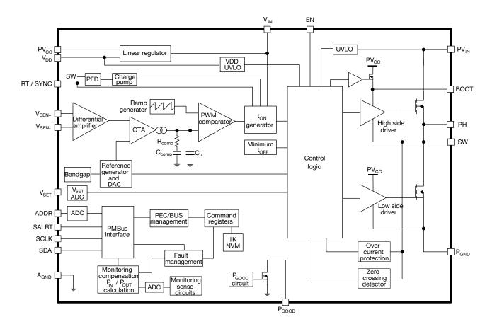
Fig. 4 - Functional Block Diagram
