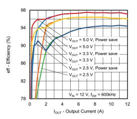
Fig. 2 - SiC454 Efficiency Curve
