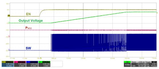
Fig. 12 - Startup with EN, No Load (1 ms/div)
