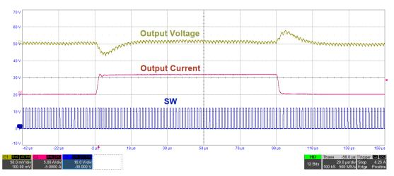
Fig. 22 - Load Step between 0 A and 6 A in CCM (20 µs/div)
