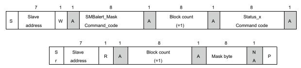
Fig. 10 - Retrieving the SMBALSER\_MASK Setting for a Given Status Register
