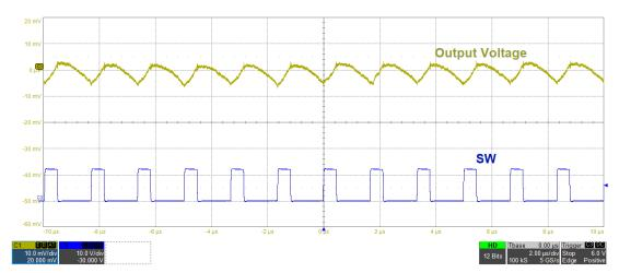
Fig. 25 - Steady State, No Load in CCM (2 µs/div)
