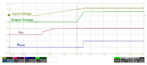
Fig. 11 - Startup with V<sub>IN</sub>, No Load (10 ms/div)
