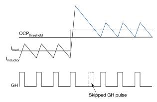
Fig. 7 - Over-Current Protection Illustration
