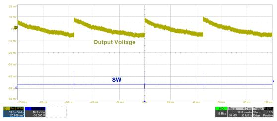
Fig. 27 - Steady State, No Load in DCM (20 ms/div)
