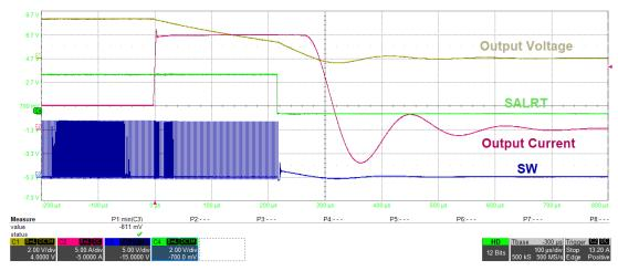
Fig. 21 - Overcurrent Protection (100 µs/div)
