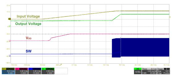
Fig. 15 - 1.5 V Pre-biased Startup with V<sub>IN</sub>, No Load (5 ms/div)
