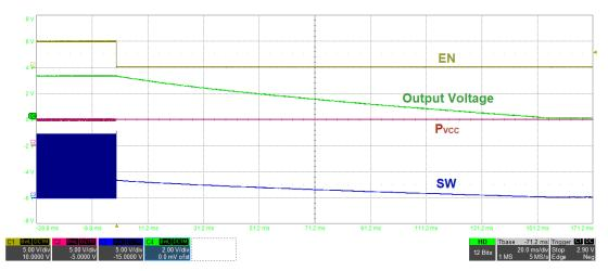
Fig. 17 - Shutdown with EN, No Load (20 ms/div)
