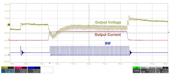
Fig. 24 - Load Step between 0 A and 6 A in DCM (20 µs/div)
