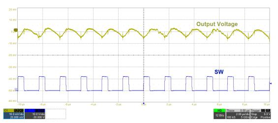
Fig. 28 - Steady State, 12 A Load (2 µs/div)
