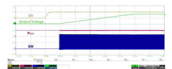
Fig. 14 - Startup with EN, 12 A Load (5 ms/div)
