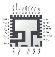
Fig. 3 - Pin Configuration - Top View
