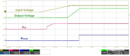
Fig. 13 - Startup with VIN, 12 A Load (5 ms/div)
