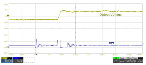
Fig. 26 - Steady State, No Load in DCM (2 µs/div)
