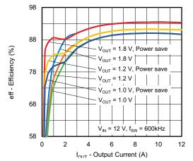
Fig. 29 - SiC454 Efficiency Curve
