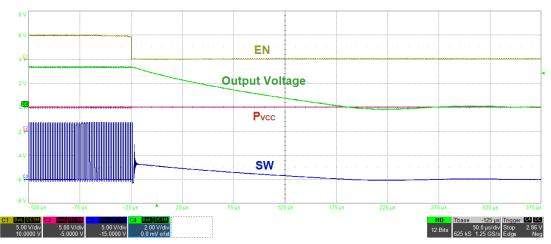
Fig. 19 - Shutdown with EN, 12 A Load (50 µs/div)
