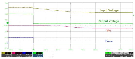
Fig. 18 - Shutdown with V<sub>IN</sub>, 12 A Load (100 ms/div)
