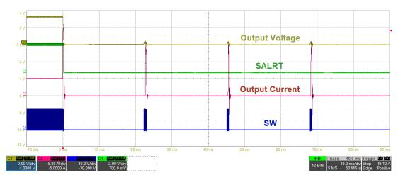
Fig. 20 - Overcurrent Protection (10 ms/div)
