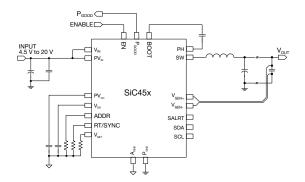
Fig. 1 - Typical Application Circuit
