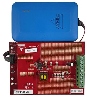
Fig. 3 - EVB Kit showing part number of SiC451EVB-KIT-A
