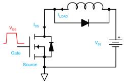
Fig. 6 - Simplified Inductive Turn-On Circuit
