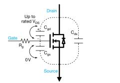
Fig. 5 - Gate Capacitances with Initial Voltages
