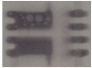
Fig. 15 - Best Case Soldering
