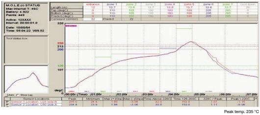
Fig. 12 - RSS Profile for Lead (Pb)-free Solder Paste
