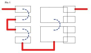
Fig. 10 - Component Modification for Daisy Chain Connection
