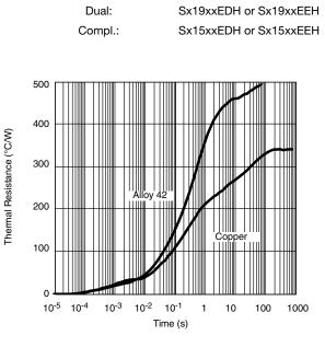
Fig. 4 Dual SC70-6 Thermal Performance on EVB
