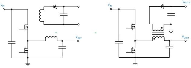
Fig. 2 - An isolated synchronous buck converter generating two outputs
