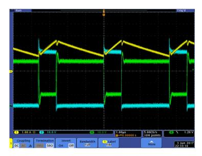
Fig. 6 - Waveform with no load on Iso +5 and 2 A on main +12 at 45  $V_{\mbox{IN}}$
