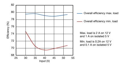
Fig. 9 - Efficiency over the input voltage range and load range (includes secondary switching regulator, U10)
