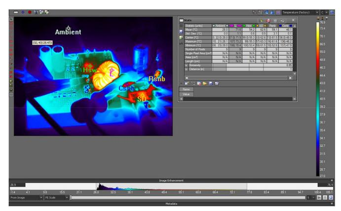
Fig. 12 - Thermal image at 55 VINPUT and a full load on both outputs
