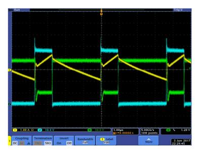
Fig. 7 - Waveform with a full load (1 A) on Iso +5 and 0 A on main +12 at 45  $\mathrm{V}_{\mathrm{IN}}$
