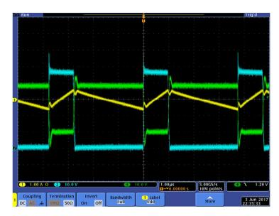
Fig. 5 - Waveform with no load on Iso +5 and 0 A on main +12 45  $V_{\text{IN}}$
