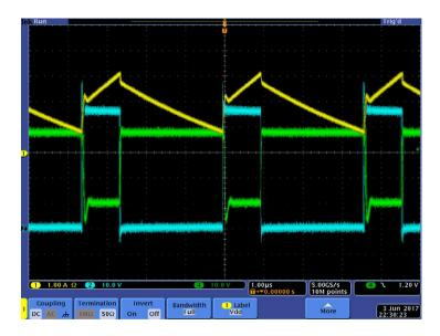
Fig. 8 - Waveform with a full load (1 A) on Iso +5 and 2 A on main +12 45  $V_{\rm IN}$
