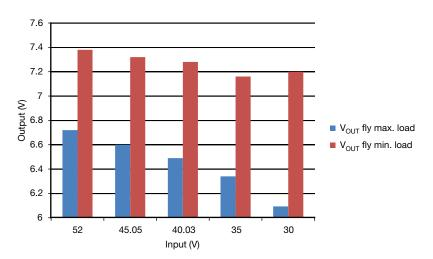
Fig. 11 - Flyback output voltage regulation on C18 over loading on all outputs and line voltage
