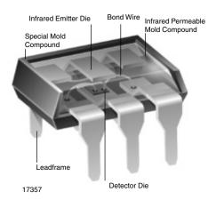
Fig. 2 - Face to Face Construction Principle
