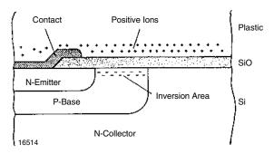
Fig. 3 - Function of Parasitic Field Effect Transistor as a Result of Failure (Latch-up) in the Phototransistor of Couplers
