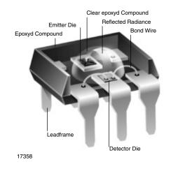
Fig. 1 - Coplanar Construction Principle
