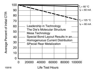
Fig. 4 - Degradation under Typical Operating Conditions
