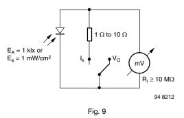
The light source used for the light measurements is a calibrated incandescent tungsten lamp with no filters.
