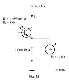
To measure collector emitter saturation voltage,  $V_{CEsat}$ , the device is illuminated and a constant collector current is passed through. The magnitude of this current is adjusted below the level of the minimum light current,  $I_{ca\ min}$ , for the same illuminance (figure 13). The saturation voltage of the phototransistor (approximately 100 mV) is then measured on a high impedance voltmeter.
