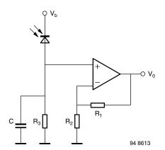
Fig. 23 - RC-Loaded Photodiode with Voltage Amplifier
