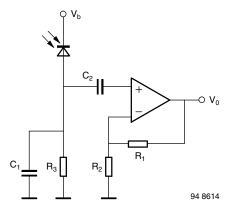
Fig. 24 - AC-Coupled Amplifier Circuit
