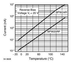
Fig. 18 - Reverse Dark Current vs. Temperature
