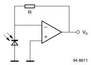
Fig. 21 - Transimpedance Amplifier, Current to Voltage Converter, Short Circuit Mode
