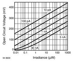
Fig. 19 - Open Circuit Voltage vs. Irradiance, Parameter: Dark Reverse Current, BPW20RF
