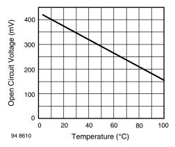
Fig. 20 - Open Circuit Voltage vs. Temperature, BPW46
