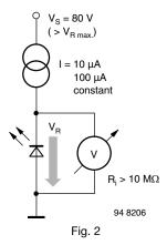
For most devices,  $V_R$  is specified at 10  $\mu A$  reverse current. In this case either a high impedance voltmeter has to be used, or current consumption of DVM has to be calculated and added to the specified current. A second measurement step will then give correct readings.
