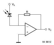
Fig. 22 - Transimpedance Amplifier, Current to Voltage Converter, Reverse Biased Photodiode
