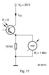
The same circuit is used for collector light current,  $l_{ca}$ , measurements (figure 12). The optical axis of the device is aligned to an incandescent tungsten lamp with no filters, producing a CIE illuminance A of 100 lx or 1000 lx with a color temperature of  $T_f = 2856$  K. Alternatively an IR irradiance by a GaAs diode can be used (refer to the photovoltaic cells and photodiodes section). Note that a lower sampling resistor is used, in keeping with the higher current involved.
