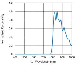
Fig. 14 - IR Channel Response
