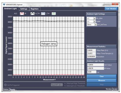
Fig. 15 - Measurement Results With a Halogen Lamp at About 1000  $\mbox{Ix}$
