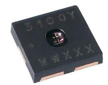
The high sensitvity of 0.0034 lx/counts allows the sensor to be placed behind very dark cover glasses that will dramatically reduce the total light reaching it. The sensor will also work behind clear cover glass, because even high illumination - such as daylight and all indoor lights - will not saturate the device and read-outs up to 228 klx are possible.
