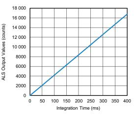
Fig. 12 - Linearity of the Integration Time
