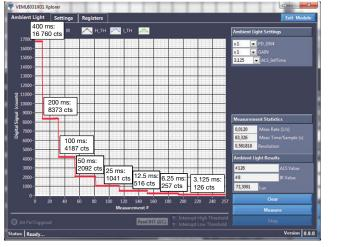
Fig. 11 - Linearity of Integration Times
