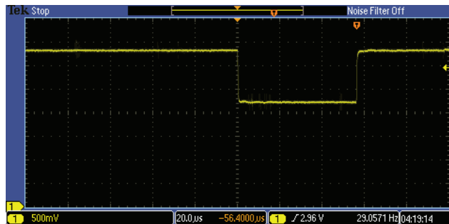
Fig. 14 - Proximity VCSEL Pulse for 1T
