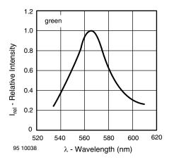
Fig. 8 - Relative Intensity vs. Wavelength
