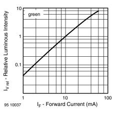
Fig. 7 - Relative Luminous Intensity vs. Forward Current
