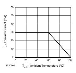
Fig. 1 - Forward Current vs. Ambient Temperature for InGaN
