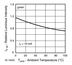
Fig. 5 - Relative Luminous Intensity vs. Ambient Temperature
