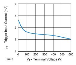
Fig. 12 - Trigger Current vs.  $V_{\text{LOAD}}$
