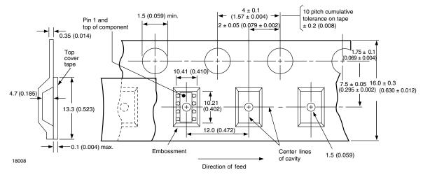
Fig. 16 - Tape and Packing (1000 pieces on reel)
