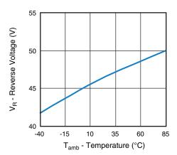
Fig. 5 - Reverse Voltage vs. Temperature
