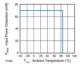
Fig. 1 - Power Dissipation vs. Temperature
