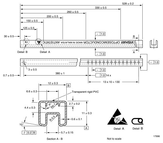
Fig. 13 - Shipping Tube Specifications for DIP Packages
