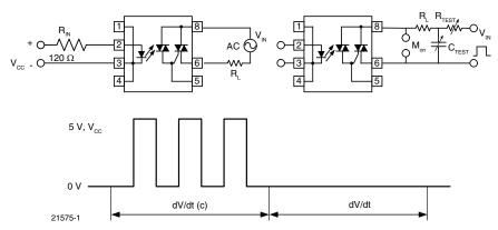
Fig. 3 - dV/dt Test Circuit
