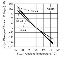
Fig. 9 - Change of Forward Voltage vs. Ambient Temperature
