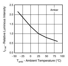
Fig. 7 - Relative Luminous Intensity vs. Ambient Temperature
