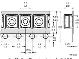
Fig. 10 - Tape Dimensions in mm for PLCC-2
