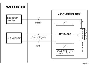
Figure 5. Block diagram of the USB to IrDA interface
