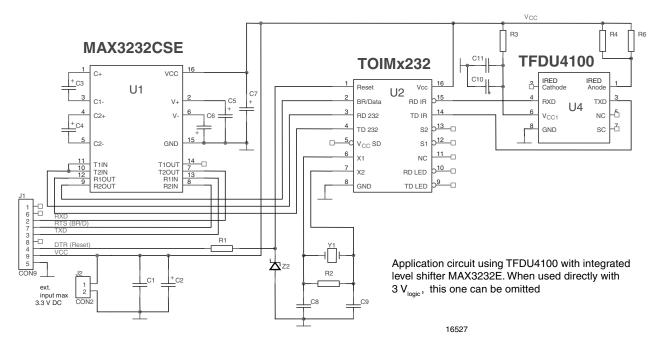
Figure 4. Application circuit using TFDU4300 with an integrated level shifter MAX3232E. When used directly with 3 V logic, this one can be omitted
