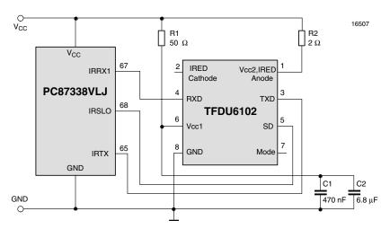
Figure 3. Application Example for TFDU6102 with NSC87338VLJ I/O
