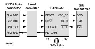
Figure 1. TOIM4232-RS232 Interface (external infrared adapter)
