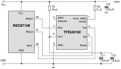
Figure 2. Application Example using NSC87108
