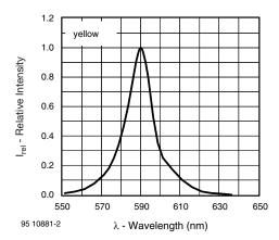
Fig. 3 - Relative Intensity vs. Wavelength
