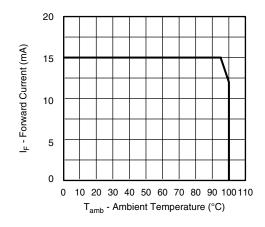
Fig. 1 - Permissible Forward Current vs. Ambient Temperature
