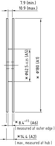
Not indicated tolerances ± 0.05 Material: black static dissipative GS15: MOQ = 5000 pcs on one reel (MOQ = minimum order quantity)
