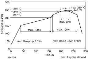
Fig. 10 - Vishay Lead (Pb)-free Reflow Soldering Profile (acc. to J-STD-020C)
