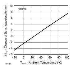
Fig. 9 - Change of Dominant Wavelength vs. Ambient Temperature
