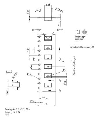
Fig. 18 - Tape for 1.9 mm Package Side View Oriented (TFBSx711TRx)
