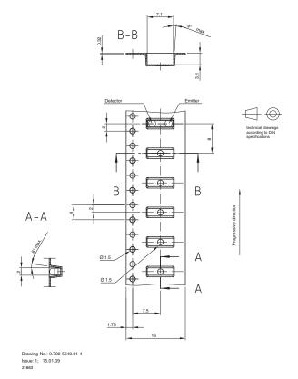
Fig. 17 - Tape for 1.6 mm Package Top View Oriented (TFBxx6xxTTx)
