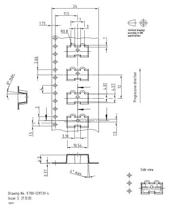
Fig. 22 - Tape for 4.0 mm Package Side View Oriented (TFDUx101TRx)
