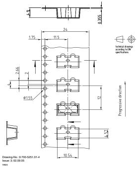
Fig. 23 - Tape for 4.0 mm Package Top View Oriented (TFDUx101TTx)
