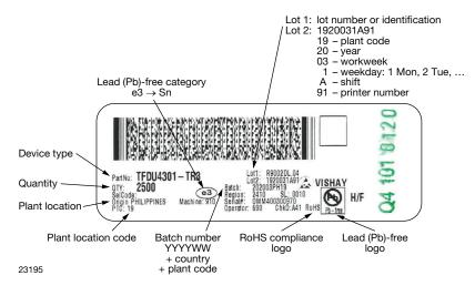
Fig. 1 - 2D Bar Code Label (according the bar code standard for 2D label PDF 417) for a Lead (Pb)-Free Device Made in Philippines, Detailed Description
