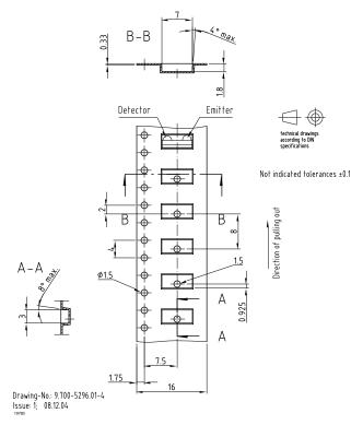
Fig. 16 - Tape for 1.6 mm Package Side View Oriented (TFBxx6xxTRx)
