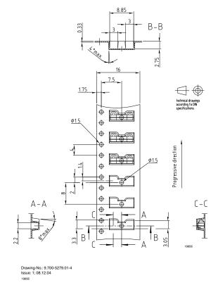
Fig. 20 - Tape for 2.5 mm Package Side View Oriented (TFDUx301TRx)
