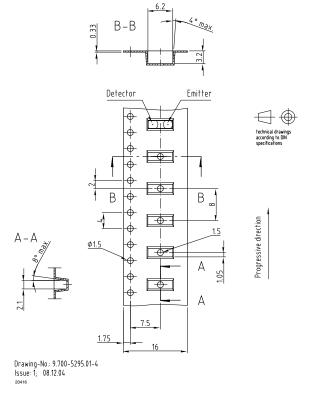
Fig. 19 - Tape for 1.9 mm Package Top View Oriented (TFBSx711TTx)
