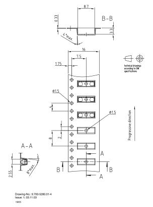
Fig. 21 - Tape for 2.5 mm Package Top View Oriented (TFDUx301TTx)
