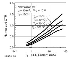
Fig. 4 - Normalized CTR vs. I<sub>F</sub> and T<sub>amb</sub>
