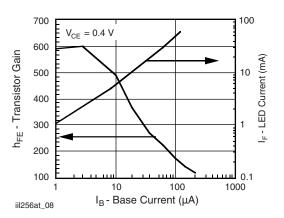
Fig. 8 - Base Current vs. I<sub>F</sub> and h<sub>FE</sub>
