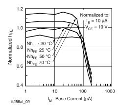
Fig. 9 - Normalized hFE vs. Base Current and Temperature
