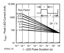
Fig. 3 - Peak LED Current vs. Duty Factor, t
