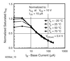
Fig. 10 - Normalized Saturated h<sub>FE</sub> vs. Base Current
