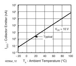
Fig. 12 - Collector Emitter Leakage Current vs. Temperature
