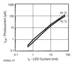
Fig. 7 - Photocurrent vs. LED Current
