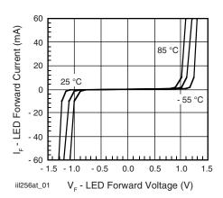
Fig. 1 - LED Forward Current vs. Forward Voltage
