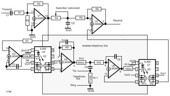
Fig. 6 - 2 to 4 Wire Optically Coupled Hybrid Norton Amplifier Configuration
