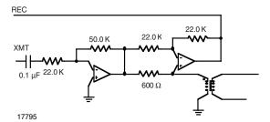
Fig. 2 - 2 to 4 Wire Electronic Hybrid
