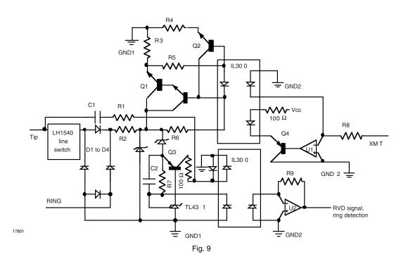
A 1 kHz transmit signal suppression of - 36 dB was measured on the bench. Both of these optical hybrids derive their power from the telco line through a voltage dropping network connected after the off/hook switch. The circuits were evaluated with 5 V to 9 V supply voltages.
