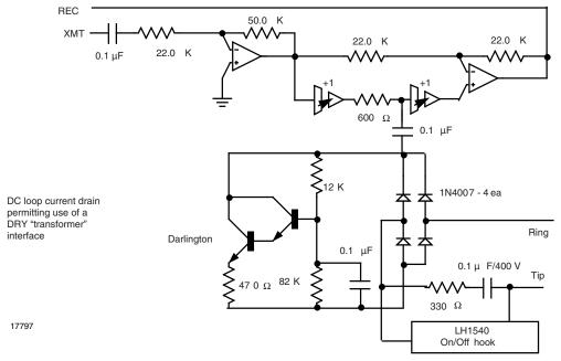
Fig. 4 - 2 to 4 Wire Hybrid Optically Isolated Transformer
