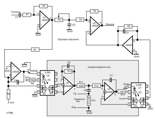
Fig. 5 - 2 to 4 Wire Optically Coupled Hybrid Norton/Thevenin Amplifier
