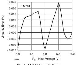
Fig. 1 - LM201 Linearity Error
