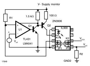
Fig. 15 - Shunt Voltage Regulator
