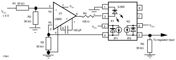
Fig. 10 - + 5 V Isolated Feedback Amplifier
