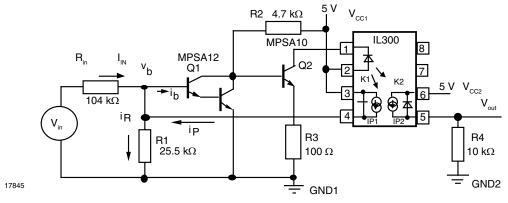
Fig. 2 - Discrete Isolation Amplifier
