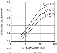
Fig. 4 - Normalized LED Efficiency
