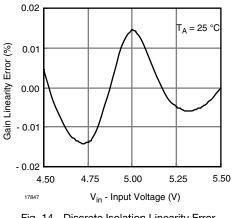
Fig. 14 - Discrete Isolation Linearity Error
