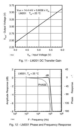
This feedback circuit offers linearity and gain accuracy of  $\pm 0.02$  % over a 4.0 V to 6.0 V input (figure 13).
