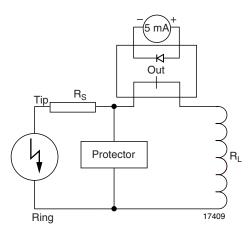
Fig. 1 - Test Setup with Protector across Tip to Ring
