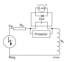
Fig. 2 - Test Setup with Protector across SSR Contacts
