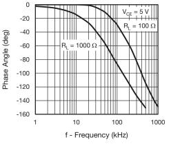
Fig. 17 - Phase Angle vs. Frequency
