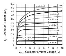
Fig. 11 - Collector Current vs. Collector Emitter Voltage (non-saturated)
