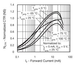
Fig. 15 - Normalized CTR (non-saturated) vs. Forward Current (I<sub>F</sub>)
