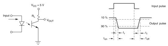
Fig. 8 - Test Circuit and Switching Waveforms
