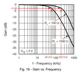
The frequency cut-off graph of figure 15 provides information regarding the highest effective frequency of a small AC signal that can be transmitted through the optocoupler. It is actually the frequency at which the output signal reaches half the amplitude, which is defined at -3 dB. The different curves show different load resistances.
