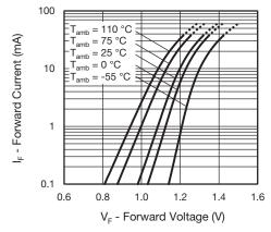
Fig. 10 - Emitter Diode Forward Current vs. Forward Voltage
