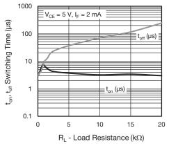
Fig. 18 - Switching Time vs. Load Resistance
