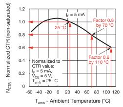
Fig. 14 - Normalized CTR (non-saturated) vs. Ambient Temperature
