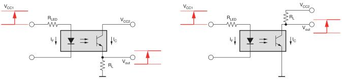
Fig. 13 - Optocoupler in Common Collector C-C (left) and Common Emitter C-E (right) Configurations
