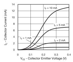
Fig. 12 - Collector Current vs. Collector-Emitter Voltage (saturated)
